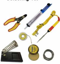
Soldering kit is used to form a permanent connection between electronic components. The metal to be soldered is heated with a soldering iron and then solder is melted into the connection. Only the solder melts, not the parts that are being soldered.
