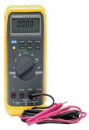
A DMM is an electronic measuring instrument that combines several measurement functions in one unit. A typical multimeter can measure voltage, current, and resistance.
